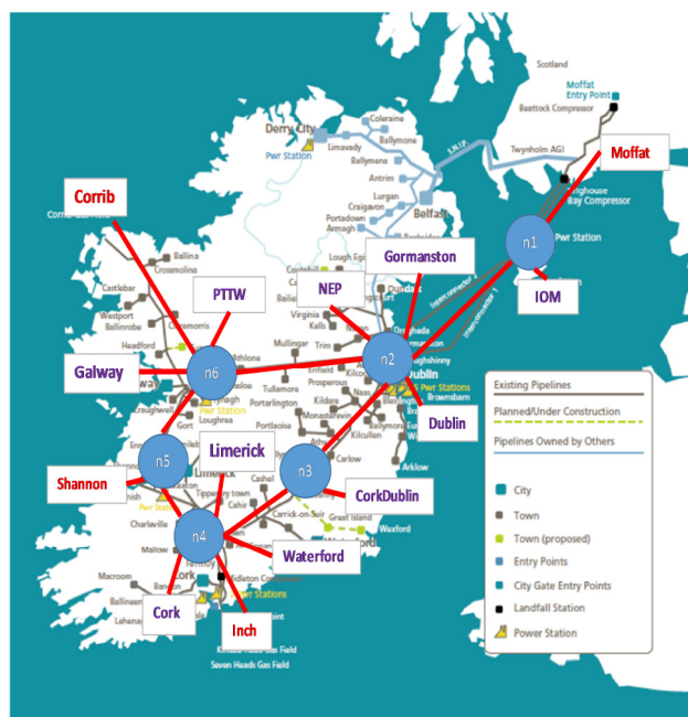
Figure 1: CEPA's Stylised Representation of the Gas Network (for the Virtual Point Approach)
