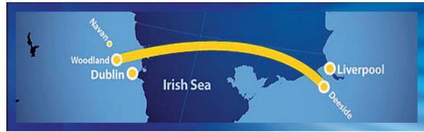
The East-West Interconnector (EWIC), currently under construction with a due operational date of 2012, will connect the electricity system in Ireland with the UK via a 260km subsea and underground cable. It will have a capacity of 500 MW and will be able to transport power in both directions. At a cost of €600 million, it is estimated to bring benefits to Ireland of over €1 billion over its 30 year economic life time. Some of the benefits are:
