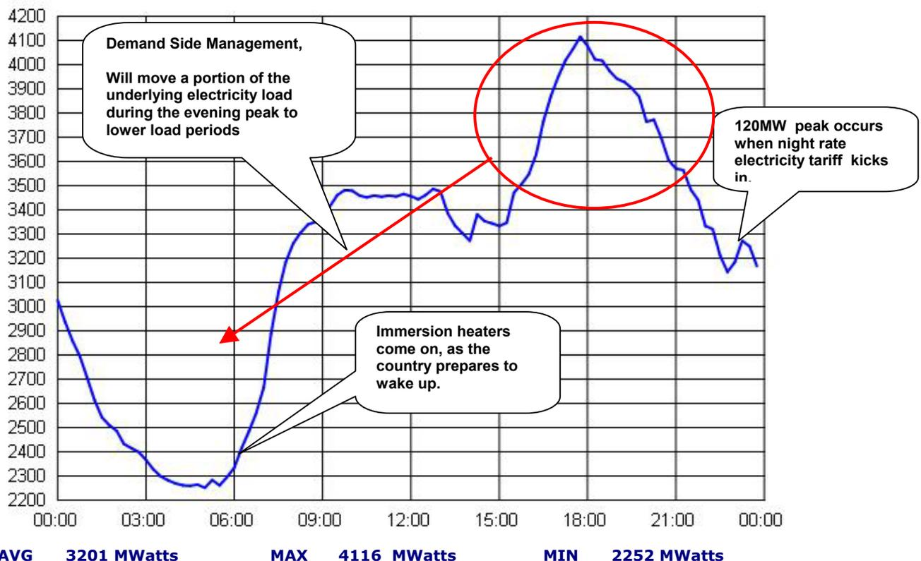
As can be seen from the graphic above, there is almost 1000 MWatts difference between the peak and average load.
